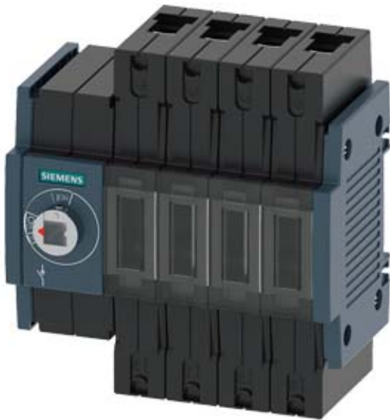
SWITCH-DISCONNECTOR 63A, FRAME SIZE 1, 4-POLE FRONT OPERATING LEFT BASIC UNIT WITHOUT HANDLE BOX TERMINAL
