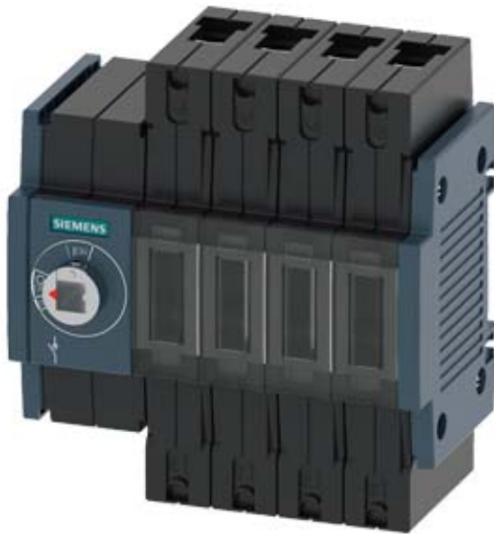
SWITCH-DISCONNECTOR 16A, FRAME SIZE 1, 4-POLE FRONT OPERATING LEFT BASIC UNIT WITHOUT HANDLE BOX TERMINAL
