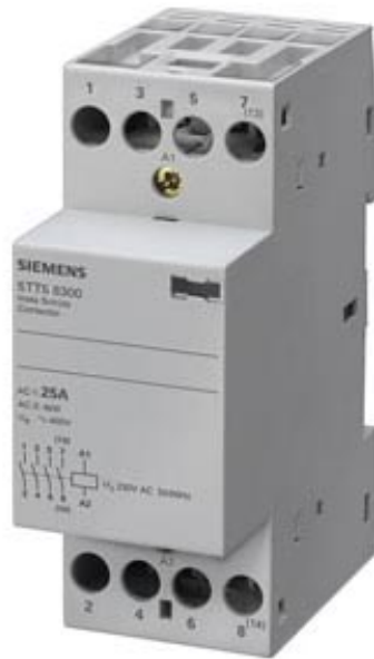
INSTA CONTACTOR WITH 4 MAKE CONTACTS CONTACT FOR 230, 400 V AC, 25 A TRIGGERING 24 V AC
