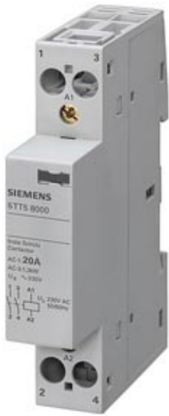
INSTA CONTACTOR WITH 1 MAKE AND 1 BREAK CONTACT CONTACT FOR 230, 400 V AC, 20 A TRIGGERING 230 V AC
