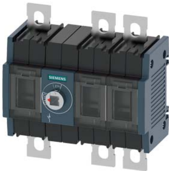
SWITCH-DISCONNECTOR 80A, FRAME SIZE 2, 3-POLE FRONT OPERATING CENTER BASIC UNIT WITHOUT HANDLE FLAT TERMINAL INCL. PHASE BARRIERS
