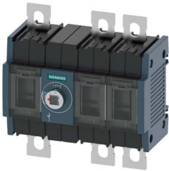
SWITCH-DISCONNECTOR 200A, FRAME SIZE 2, 3-POLE FRONT OPERATING CENTER BASIC UNIT WITHOUT HANDLE FLAT TERMINAL INCL. PHASE BARRIERS
