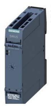
TIME RELAY, ELECTRONIC, WITH STAR-DELTA FUNCTION, 1 CONTACTOR DELAYED, 1 CONTACTOR NON-DELAYED, 1 TIME SET. RANGE 3...60S, 12...240V AC/DC AT AC 50/60HZ, LED, SPRING-LOADED TERMINAL (PUSH-IN)
