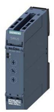
TIME RELAY, MULTI-FUNCTION, 2 CO CONT., 27 FUNCT., 15 TIME SET. RANGES (1, 3, 10, 30, 100) (S/MIN/HR), 400-440V AC AT AC 50/60HZ, LED, SPRING-LOADED TERMINAL (PUSH-IN)
