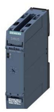
TIME RELAY, ELECTRONIC, WITH STAR-DELTA FUNCTION, 1 CONTACTOR DELAYED, 1 CONTACTOR NON-DELAYED, 1 TIME SET. RANGE 3...60S, 200...240V AC AND 380...440V AC SCREW **TERMINAL**
