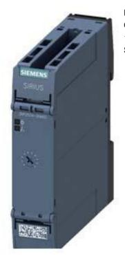
TIME RELAY, ELECTRONIC, WITH STAR-DELTA FUNCTION, 1 CONTACTOR DELAYED, 1 CONTACTOR NON-DELAYED, 1 TIME SET. RANGE 1...20S, 200...240V AC AND 380...440V AC LED, SPRING-LOADED TERMINAL (PUSH-IN)
