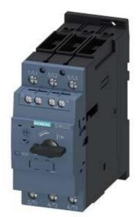
CIRCUIT BREAKER, SIZE S2, FOR MOTOR PROTECTION, CLASS 10, A-RELEASE 22...32A, N-RELEASE 416A, SCREW TERMINAL, STANDARD BREAKING CAPACITY W. TRANSV. AUX. SWITCH 1NO+1NC
