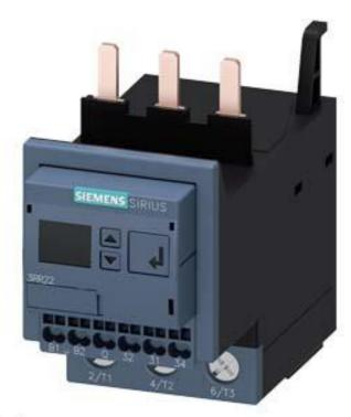
MONITORING RELAY ATTACHABLE TO CONTACTOR 3RT2. SIZE S2 STANDARD, DIGITAL ADJUSTABLE APPARENT/ACTIVE CURRENT MONIT. 8 - 80A, 20-400 HZ, 3-PHASE SUPPLY 24 V AC/DC 1 CO CONTACT, 1 SEMICOND. FOR ALARM AND WARNING MONITORING FOR CURRENT OVERSHOOT/UNDERSHOOT PHASE FAILURE, WIRE BREAK PHASE SEQUENCE FAULT CURRENT BLOCKING CURRENT WARNING AND ALARM THRESHOLDS WITH OR W/O ERROR LOG ONDELAY 0-99 S SPURIOUS PEAK SUPPR.0-30 S BREAK AFTER FAULT 0-300 MIN SPRING-LOADED CONNECTION
