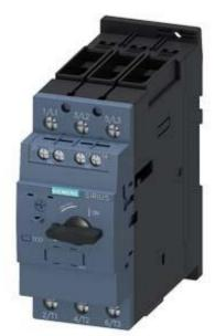
CIRCUIT BREAKER, SIZE S2, FOR MOTOR PROTECTION, CLASS 10, A-RELEASE 28...36 A, N-RELEASE 520A, SCREW TERMINAL, STANDARD BREAKING CAPACITY, W. TRANSV. AUXILIARY SWITCH 1NO+1NC
