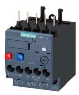
OVERLOAD RELAY 1.8...2.5 A FOR MOTOR PROTECTION SZ S00, CLASS 10, F. MOUNTING ONTO CONTACTOR MAIN CIRCUIT: SCREW TERMINAL AUX. CIRCUIT: SCREW TERMINAL MANUAL-AUTOMATIC-RESET
