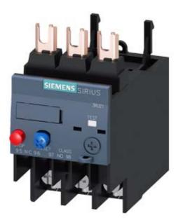
OVERLOAD RELAY 30...36 A FOR MOTOR PROTECTION SZ S0, CLASS 10, F. MOUNTING ONTO CONTACTOR MAIN CIRCUIT: RING CABLE LUG AUX. CIRCUIT: RING CABLE LUG MANUAL-AUTOMATIC-RESET
