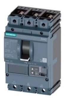
CIRCUIT BREAKER 3VA2 IEC FRAME 250 BREAKING CAPACITY CLASS M ICU=55KA @ 415 V 3POLE, LINE PROTECTION ETU860, LSIG, IN=160A OVERLOAD PROTECTION IR=64A ...160A SHORT CIRCUIT PROTECTION ISD=0,6..10X IN, II=1,5..12X IN NEUTRAL PROTECTION OPTIONAL WITH EXT. CT,UPTO 160% GROUNDFAULT, SWITCHABLE IG=0,2... 1 X IN, TG=0,050,8MS BUSBAR CONNECTION
