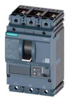
CIRCUIT BREAKER 3VA2 IEC FRAME 250 BREAKING CAPACITY CLASS M ICU=55KA @ 415 V 3POLE, LINE PROTECTION ETU850, LSI, IN=250A OVERLOAD PROTECTION IR=100A ...250A SHORT CIRCUIT PROTECTION ISD=0,6..10X IN, II=1,5..10X IN NEUTRAL PROTECTION OPTIONAL WITH EXT. CT,UPTO 160% BUSBAR CONNECTION
