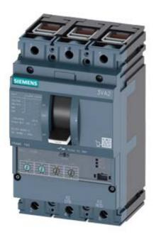
CIRCUIT BREAKER 3VA2 IEC FRAME 160 BREAKING CAPACITY CLASS M ICU=55KA @ 415 V 3POLE, LINE PROTECTION ETU350, LSI, IN=100A OVERLOAD PROTECTION IR=40A ...100A SHORT CIRCUIT PROTECTION ISD=1,5... 10 X IR, II=12 X IN CABLE CONNECTION
