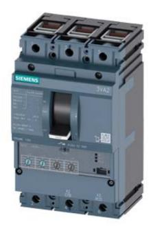
CIRCUIT BREAKER 3VA2 IEC FRAME 160 BREAKING CAPACITY CLASS M ICU=55KA @ 415 V 3POLE, LINE PROTECTION ETU330, LIG, IN=100A OVERLOAD PROTECTION IR=40A ...100A SHORT CIRCUIT PROTECTION II=1,5...12 X IN GROUNDFAULTPROTECTION IG=0,2... 1 X IN, TG=0,1/0,3MS CABLE CONNECTION
