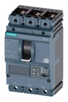
CIRCUIT BREAKER 3VA2 IEC FRAME 160 BREAKING CAPACITY CLASS M ICU=55KA @ 415 V 3POLE, LINE PROTECTION ETU560, LSIG, IN=160A OVERLOAD PROTECTION IR=64A ...160A SHORT CIRCUIT PROTECTION ISD=0,6..10X IN, II=1,5...10X IN NEUTRAL PROTECTION OPTIONAL WITH EXT. CT,UPTO 160% GROUNDFAULT, SWITCHABLE IG=0,2... 1 X IN, TG=0,050,8MS BUSBAR CONNECTION
