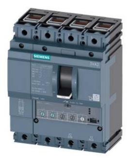
CIRCUIT BREAKER 3VA2 IEC FRAME 160 BREAKING CAPACITY CLASS M ICU=55KA @ 415 V 4POLE, LINE PROTECTION ETU330, LIG, IN=160A OVERLOAD PROTECTION IR=64A ...160A SHORT CIRCUIT PROTECTION II=1,5...10 X IN NEUTRAL PROTECTION ADJUSTABLE(OFF,50%,100%) GROUNDFAULTPROTECTION IG=0,2... 1 X IN, TG=0,1/0,3MS CABLE CONNECTION
