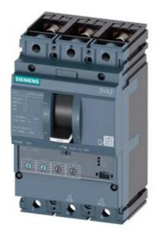
CIRCUIT BREAKER 3VA2 IEC FRAME 160 BREAKING CAPACITY CLASS M ICU=55KA @ 415 V 3POLE, LINE PROTECTION ETU330, LIG, IN=160A OVERLOAD PROTECTION IR=64A ...160A SHORT CIRCUIT PROTECTION II=1,5...10 X IN GROUNDFAULTPROTECTION IG=0,2... 1 X IN, TG=0,1/0,3MS BUSBAR CONNECTION
