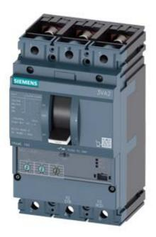
CIRCUIT BREAKER 3VA2 IEC FRAME 160 BREAKING CAPACITY CLASS M ICU=55KA @ 415 V 3POLE, LINE PROTECTION ETU320, LI, IN=160A OVERLOAD PROTECTION IR=64A ...160A SHORT CIRCUIT PROTECTION II=10 X IN BUSBAR CONNECTION
