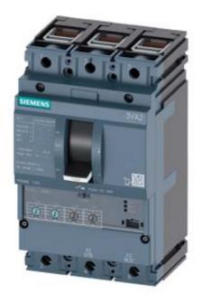
CIRCUIT BREAKER 3VA2 IEC FRAME 100 BREAKING CAPACITY CLASS M ICU=55KA @ 415 V 3POLE, LINE PROTECTION ETU330, LIG, IN=63A OVERLOAD PROTECTION IR=25A ...63A SHORT CIRCUIT PROTECTION II=1,5...12 X IN GROUNDFAULTPROTECTION IG=0,2... 1 X IN, TG=0,1/0,3MS CABLE CONNECTION
