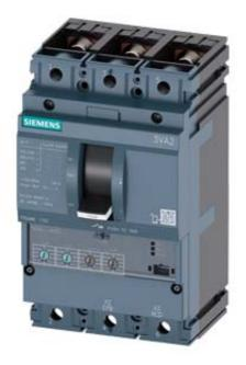
CIRCUIT BREAKER 3VA2 IEC FRAME 100 BREAKING CAPACITY CLASS M ICU=55KA @ 415 V 3POLE, LINE PROTECTION ETU350, LSI, IN=100A OVERLOAD PROTECTION IR=40A ...100A SHORT CIRCUIT PROTECTION ISD=1,5... 10 X IR, II=12 X IN BUSBAR CONNECTION
