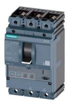
CIRCUIT BREAKER 3VA2 IEC FRAME 100 BREAKING CAPACITY CLASS M ICU=55KA @ 415 V 3POLE, LINE PROTECTION ETU330, LIG, IN=100A OVERLOAD PROTECTION IR=40A ...100A SHORT CIRCUIT PROTECTION II=1,5...12 X IN GROUNDFAULTPROTECTION IG=0,2... 1 X IN, TG=0,1/0,3MS BUSBAR CONNECTION
