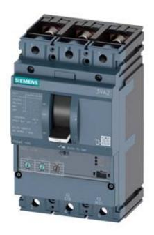
CIRCUIT BREAKER 3VA2 IEC FRAME 100 BREAKING CAPACITY CLASS M ICU=55KA @ 415 V 3POLE, LINE PROTECTION ETU320, LI, IN=100A OVERLOAD PROTECTION IR=40A ...100A SHORT CIRCUIT PROTECTION II=12 X IN BUSBAR CONNECTION
