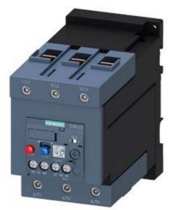
THERM. OVERLOAD RELAY 70...90 A FOR MOTOR PROTECTION SIZE S3, CLASS 10 FOR STAND-ALONE MOUNTING MAIN CIRCUIT: SCREW TERMINAL AUX. CIRCUIT: SCREW TERM. MANUAL-AUTOMATIC-RESET
