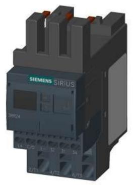
CURRENT MONITORING RELAY MOUNTABLE ON CONT. 3RT2, SZ. SO, APPARENT/ACTIVE CURR. MONIT. 4 - 40A, 20-400 HZ, 3-PH., SUPPLY 24 V DC, 1 CO CONTACT, MONITORING F. CURRENT OVER/UNDERSHOOT, CURRENT ASYMMETRY, PHASE FAILURE / WIRE BREAK, PHASE SEQUENCE, FAULT CURRENT, BLOCKING CURRENT, SWITCHING CYCLE/OP. HOURS COUNTER, WARNING/ALARM THRESHOLDS, AUTO OR MANUAL RESET ONDELAY 0-999.9 S OFF-DELAY 0-999.9 S RECLOSING DELAY 0-999.9MIN SPRING-LOADED CONNECTION
