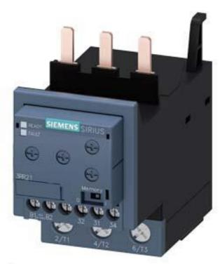
Monitoring relay, attachable to contactor 3RT2, size S2 Basic, analog adjustment Apparent current monitoring 8...80 A, 50...60 Hz, 2-phase Supply 24-240 V AC/DC 1 changeover contact Monitoring for current overshoot and undershoot Phase failure, wire break with or without fault buffer ON delay 0-60 s Spurious peak suppr. 0-30 s Switching hysteresis 6% Screw terminal
