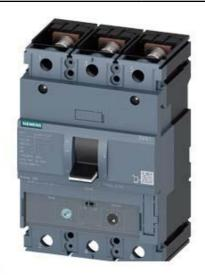
CIRCUIT BREAKER 3VA1 IEC FRAME 250 BREAKING CAPACITY CLASS S ICU=36KA @ 415 V 3-POLE, LINE PROTECTION TM240, ATAM, IN=160A OVERLOAD PROTECTION IR=112A ...160A SHORT CIRCUIT PROTECTION II=5...10 X IN BUSBAR CONNECTION
