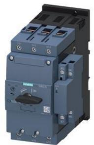
CIRCUIT-BREAKER SIZE S3, FOR MOTOR PROTECTION, CLASS 10, WITH OVERLOAD RELAY FUNCTION A-REL. 28...40 A, N-RES. 520 A, SCREW CONNECTION, INCREASED BREAKING CAPACITY
