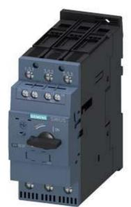
CIRCUIT BREAKER, SIZE S2, FOR MOTOR PROTECTION, CLASS 10, A-RELEASE 70..80A, N-RELEASE 1040A, SCREW TERMINAL, STANDARD BREAKING CAPACITY W. TRANSV. AUX. SWITCH 1NO+1NC
