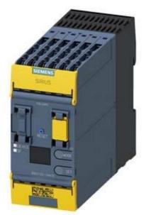
SIRIUS SAFETY RELAY BASIC UNIT 3SK2 SERIES 20 F-DI, 4 F-DQ, 2 DQ, 24 V DC PARAMETERIZABLE VIA SIRIUS SAFETY ES WIDTH 45MM SCREW TERMINALS UP TO SILCL 3 (DIN EN 62061) UP TO PERFORMANCE LEVEL E (ISO 13849-1) 3SK1 OUTPUT EXPANSIONS AND 3RM1 FAIL-SAFE MOTOR STARTER CONNECTABLE VIA DEVICE CONNECTOR
