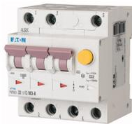
**RCD/MCB, 13A, 30mA, miniature circuit-breaker trip curve C, 3 p, residual current circuit-breaker trip characteristic: A**
