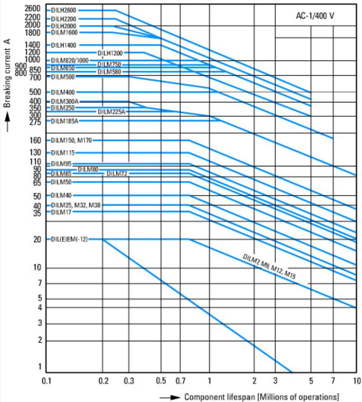
Switching duty for non-motor loads, 3-pole, 4-pole
