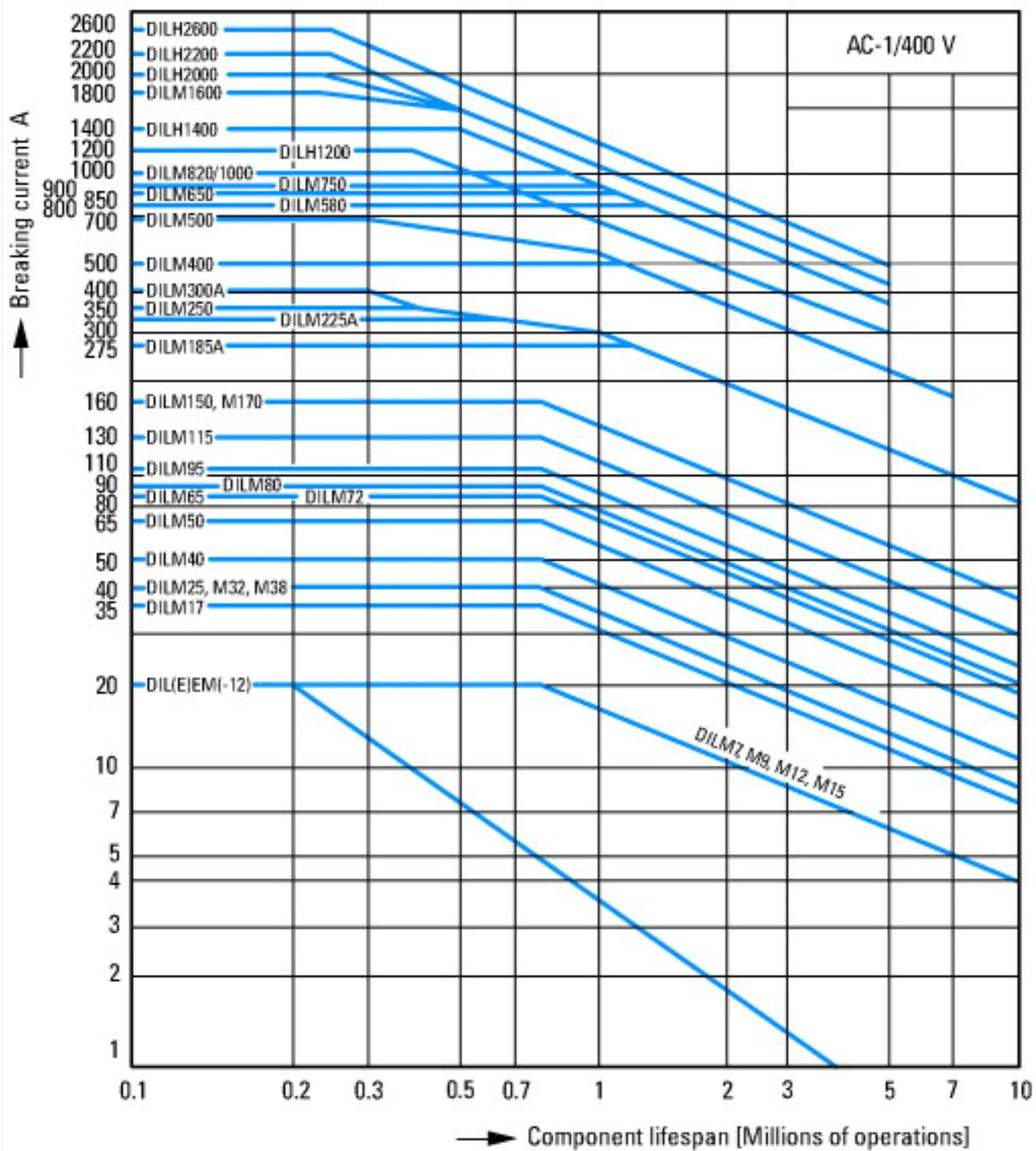
Switching conditions for 3 pole, non-motor loads
