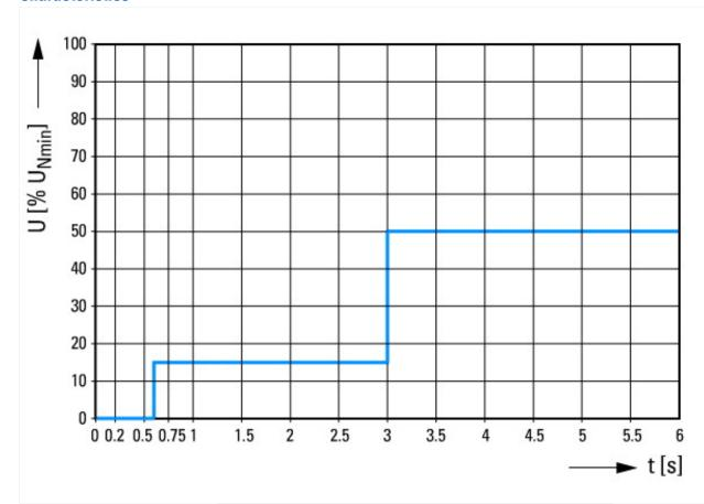
Limits for the delay times used to maintain operation in the event of voltage fluctuations.
