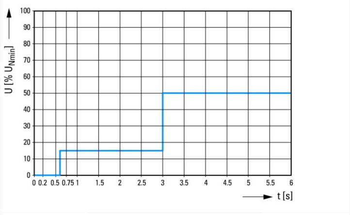
Limits for the delay times used to maintain operation in the event of voltage fluctuations.
