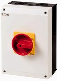
**Main switch, 3 pole, 100 A, Emergency-Stop function, Lockable in the 0 (Off) position, surface mounting**
