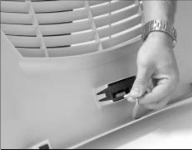
Fig. 34: Disconnect the connector from the display
