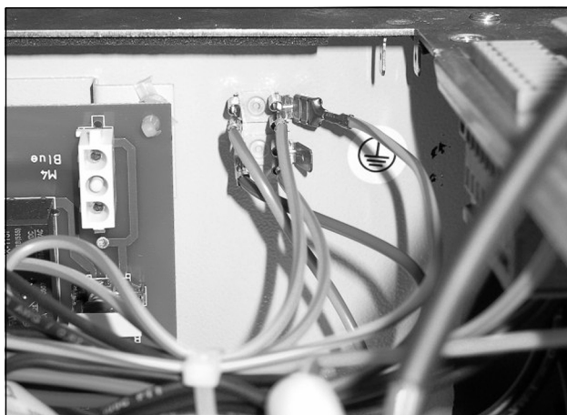
Fig. 23: Disconnect the earthing cable
