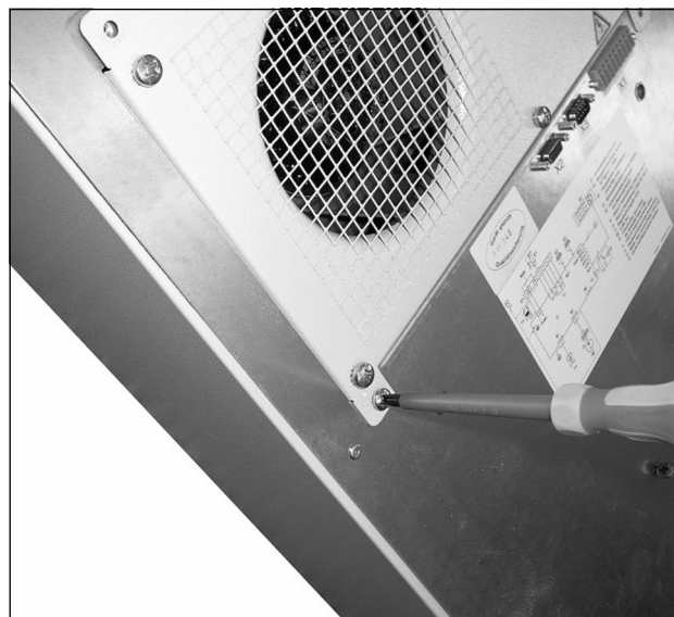
Fig. 20: Remove the fastening screws for the cover with fan
