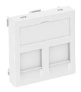
The Type A data technology support is suitable for accepting the following data connection modules: AMP TYCO (without dust protection cap): SL Series 110Connect and SL Series Toolless; Brand-Rex: modules with item numbers ending in ...JAKS000CR and ...JAKU002; Nexans: LANmark RJ45 with blue adapter clip, LANmark GG45 with metal clip.
