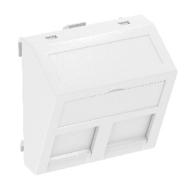
Data technology support with slanting outlet and locking slider to accept two data technology connection modules with RJ45 socket. The locking fastening is suitable for horizontal and vertical installation in the system environment. Type A has a mounting opening of  $20.10 \times 14.80$  mm and is designed for direct fastening of the data connection modules in the mounting opening.
