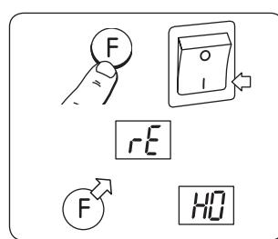
Hold in the **F** key and then switch the heater ON.
