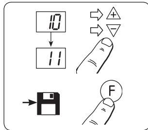
When cutback temperature is ongoing, select the new cutback temperature you desire by pressing  $\Delta$  or  $\nabla$ .
