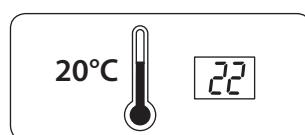
Should the actual room temperature and Neo's setting not correspond, Neo should be calibrated.
