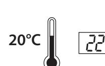
Hold down on **F** and press once on  **$\nabla$** . Release **F**. **°C** will flash 3 times and the setpoint temperature will flash. Press  $\Delta$  or  $\nabla$  until the display shows the same as the actual measured room temperature. Store by pressing **F** for 5 seconds.
