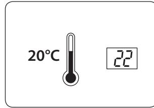
The thermostat will now work with the temperature displayed by Neo and after a period this will correspond with the actual temperature of the room. This procedure can be repeated at a later date to ensure correct calibration.
