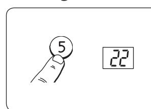
Press ⑤ for 5 seconds. The set comfort temperature will show in the display. The LED above the ⑤ key will light steady while the LED above the ⑦ key will continue flashing. You now have a temporary comfort period lasting five hours.
