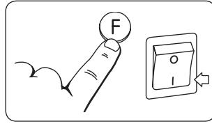
Press and hold in F and then switch on using the main power switch. Continue to press F until rE flashes in the display, then release F.
