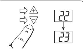
Selecting another temperature during either a comfort or cutback period, without storing it (by pressing **F** for 5 seconds), will apply only to the current period.
