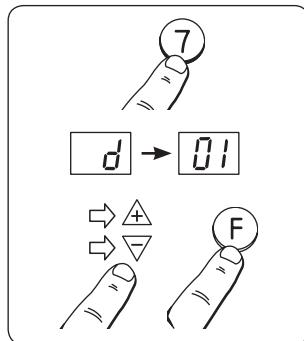
Press 7 for 5 seconds. d (days) will flash 3 times. 01 (days) will flash continuously.
