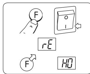
Hold in the  $\text{F}$  key and then switch the heater ON.
