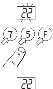
At the time the frost-safe period ends, the comfort temperature setting will flash to indicate the need for action. Press any key to make the comfort temperature display steadily and that temperature will now continue.
