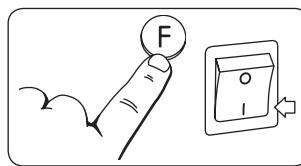
Press F and hold in and at the same time switch on using the main power switch.
