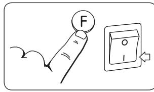
Press F and hold in and at the same time switch on using the main power switch.
