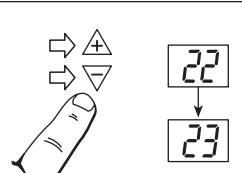
If you select another temperature during either a comfort or a cutback period, and do not save (by pressing **F** for five seconds), the new temperature will apply only to the current period.
