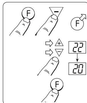
Hold down on  $\text{F}$  and press once on  $\nabla$ . Release  $\text{F}$ .  $^{\circ}\text{C}$  will flash 3 times and the setpoint temperature will flash. Press  $\Delta$  or  $\nabla$  until the display shows the same as the actual measured room temperature. Store by pressing  $\text{F}$  for 5 seconds.
