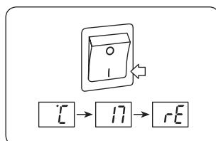
On switching heater on, the sequence °C – 17 – rE – will flash in the display.
