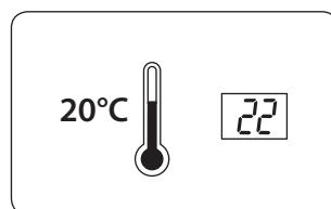
The thermostat will now work with the temperature displayed by Neo and after a period this will correspond with the actual temperature of the room. This procedure can be repeated at a later date to ensure correct calibration.
