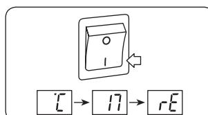
On switching heater on, the sequence °C – 17 – rE – will flash in the display.
