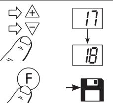
While cutback temperature is ongoing, choose the desired new cutback temperature by pressing  $\Delta$  or  $\nabla$ . Save the setting by pressing **F** more than five seconds.
