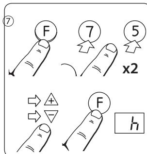
Hold down on **F** and press twice on **7**. Release **F** and **h** (hours) will flash 3 times.
