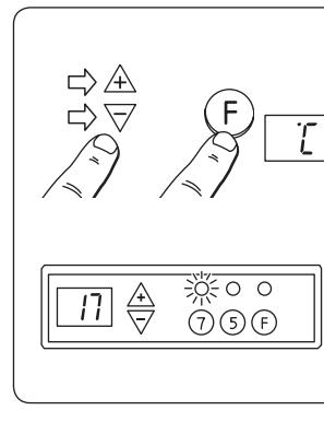
°C will flash three times and then 17 (°C) will flash continuously. With the ▲ or ▼ key select your preferred cutback temperature.
