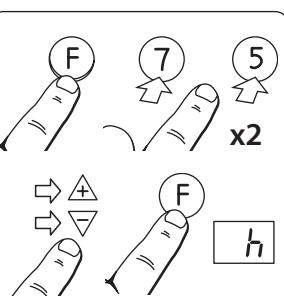
Hold down on **F** and press twice on **7** or **5**. Release **F** and **h** (hours) will flash 3 times.
