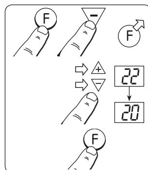
Hold down on **F** and press once on **▼**. Release **F**. **°C** will flash 3 times and the setpoint temperature will flash. Press **▲** or **▼** until the display shows the same as the actual measured room temperature. Store by pressing **F** for 5 seconds.
