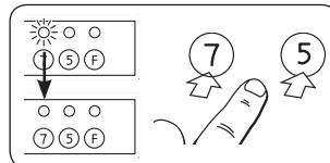
To permanently delete a temperature cutback function, press **7** or **5** until the green lamp goes out.
