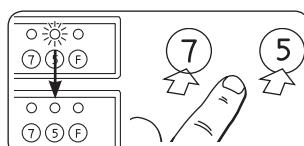
To permanently delete a temperature cutback function, press **7** or **5** until the green lamp goes out.
