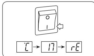
On switching heater on, the sequence °C – 17 – rE – will flash in the display. This means that the thermostat has been disconnected for a long period and needs to be restarted.
