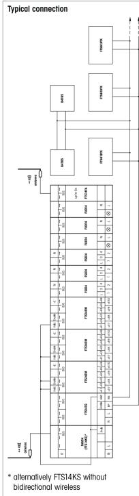
The second terminating resistor supplied with the FAM14 or FTS14KS must be plugged into the last bus user. Use the
