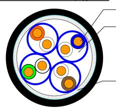
Conductor (23AWG/1 - Solid Bare Copper)
