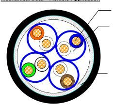
Conductor (26AWG/7 – 7x0.16mm Stranded Copper)
