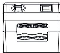
Secondary strain relief for cable with smaller cable sheath
