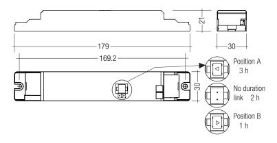
Note: LED Driver supplied with duration link in 3 hours position. Duration link must be set before battery and mains connection. The EM converterLED PRO 134 NiCd is supplied without a duration link. The duration is set to 3 hours and cannot be changed.
