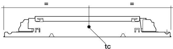
The nominal  $t_a$  and  $t_c$  point are related to the ballast life duration. The relation of  $t_c$  to  $t_a$  temperature depends also on the luminaire design. If the measured  $t_c$  temperature is approx. 5 K below  $t_c$  max.,  $t_a$  temperature should be checked and eventually critical components (e.g. ELCAP) measured. Detailed information on request.
